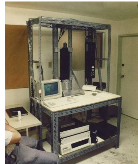
Early 3D Systems SL Prototype
